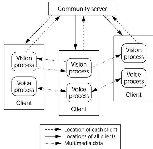
Figure 7. FreeWalk system configuration.
