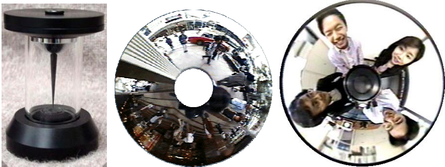
Fig. 2. Omni-Directional Vision Sensor [5]
