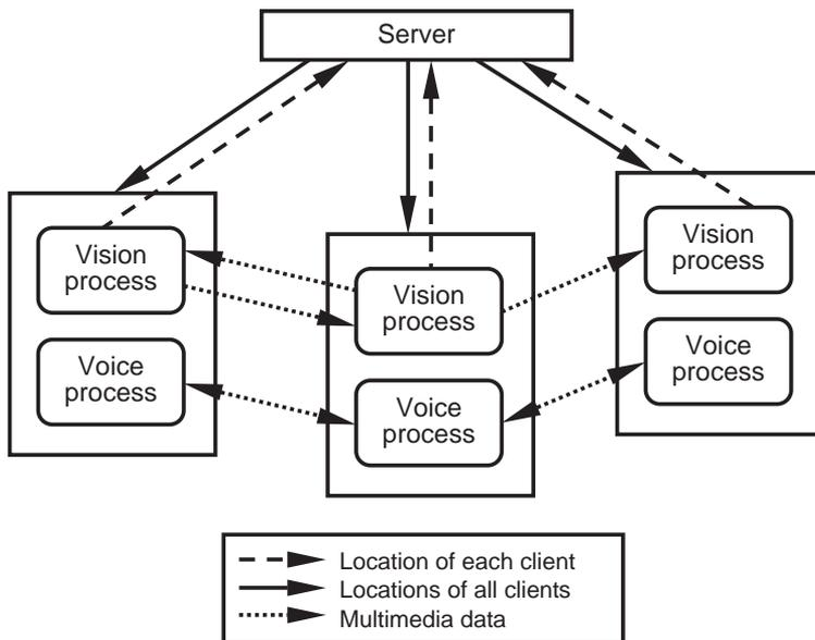
Fig. 5. FreeWalk system architecture.
