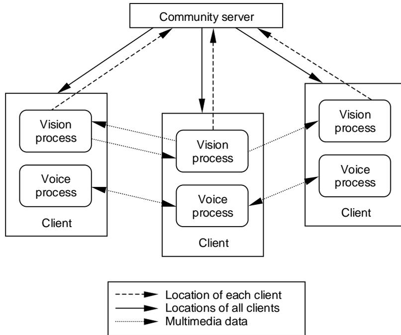
Figure 7. FreeWalk system configuration.
